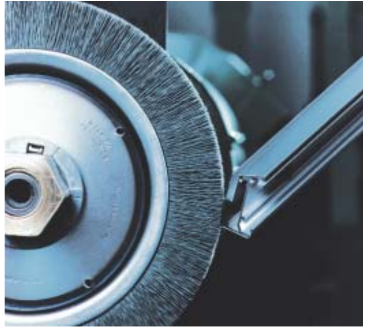
Entgraten von Aluminiumprofilen. Deburring of aluminium profiles.
