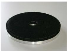
The **SoftDisc** is used for deburring using a standard abrasive disc with velcro backing. The soft backing ensures an aggressive grinding at the edges of the workpiece without applying too much pressure on the surface.
