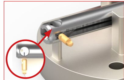
Insert new blade with cutting edges up into the blade holder. Make sure that the blade is pushed in from the line mark side.
